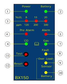
1) MAINS LED. It lights up when electrical power is connected. Initially, this LED blinks for about 1 minute and a half waiting for the check.
