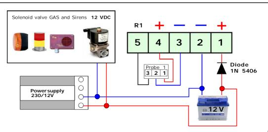
If a 12Vdc solenoid valve, which does not work well, is connected to the BX150. Direct connection of 12VDC solenoid valves or sirens to the **BX150** is not permitted. An external power unit must always be used. The BX150 M gives a **max** current of **50mA**.
