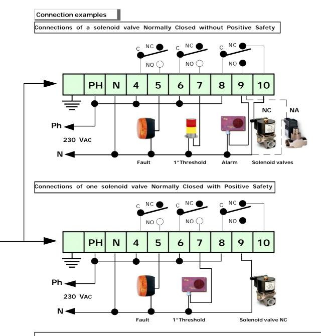
If a 12Vdc solenoid valve, which does not work well, is connected to the BX150. Direct connection of 12VDC solenoid valves or sirens to the **BX150** is not permitted. An external power unit must always be used. The BX150 M gives a **max** current **of 50mA**.
