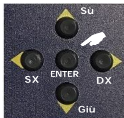
Group of navigation buttons. These buttons are used to set the operation of the control unit.
