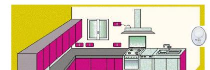
Methane and carbon monoxide gas detector max. 30 cm from the ceiling min. 1,60 from the floor
