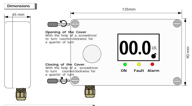
Installation and positioning of the detector
