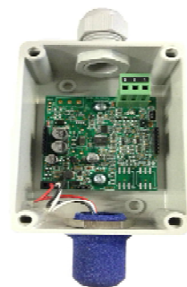
Probe with sensor reinstalled
