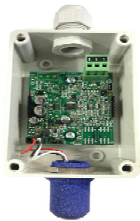
Probe with sensor to be replaced
