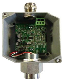
Probe with sensor to be replaced
