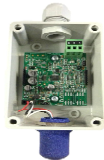
Probe with sensor remounted
