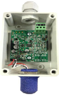
Probe with sensor to be replaced
