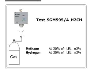
The installation of the **SGM595/A-H2CH** probe, its ordinary and extraordinary maintenance, and its out of service removal at the end of the functional life guaranteed by the manufacturer, must be carried out by authorized or specialized personnel.
